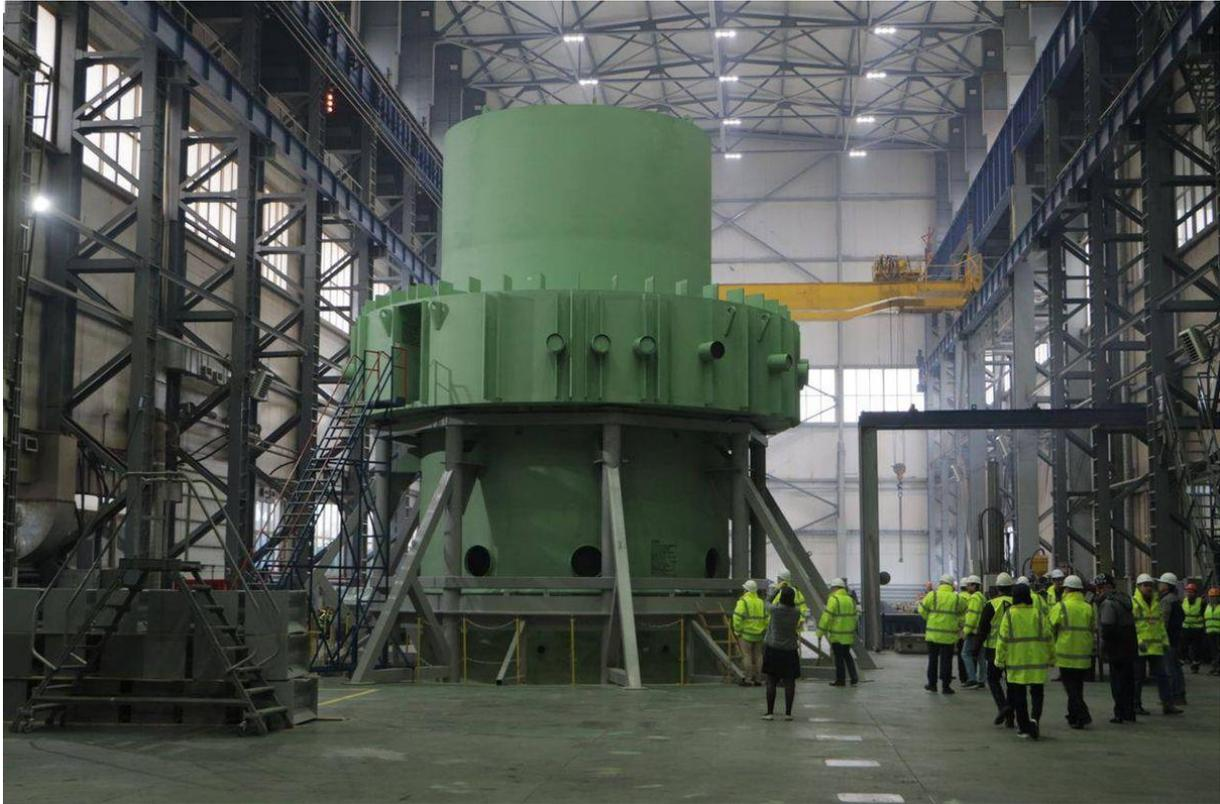
In April 2024, production of another main equipment, the reactor pressure vessel belonging to unit 5 began at the SpecStal factory of the AEM-Technologies Group, a subsidiary of Rosatom. The production plant is located in Kolpino near St. Petersburg, where typically raw materials and semi-finished products are manufactured. The production started with casting the ingots of the upper and the lower shells of the nozzle-area of the vessel, followed by the forging of those parts.
